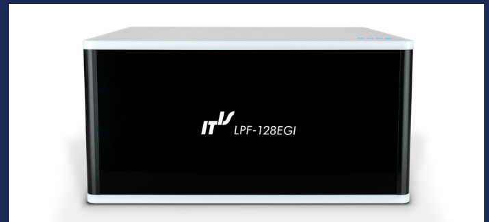
LPF-128EGI: 128-channel low-pass filter for EGI Net Amps Series
